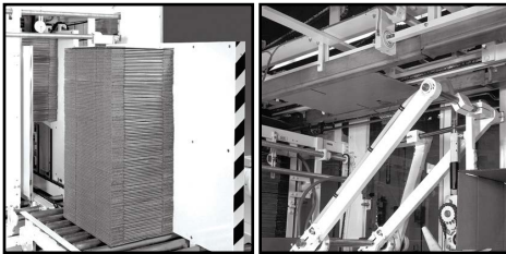
Stack of KD cases entering the FF 100 elevator KD case is delivered from elevator to opening station
