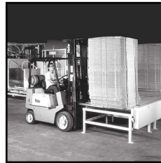
BN 200 with optional KD cases transfer to load station
