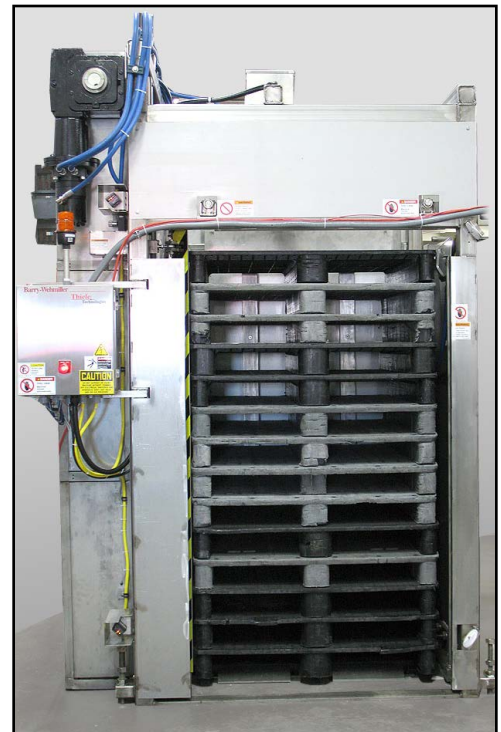
Stack of clean pallets for unloading
